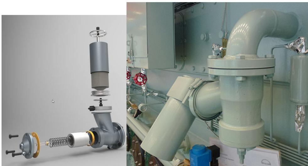
*Exploded view of a Part-Load Optimisation charge-air blow-off valve (left); and close-up on engine (right)*
